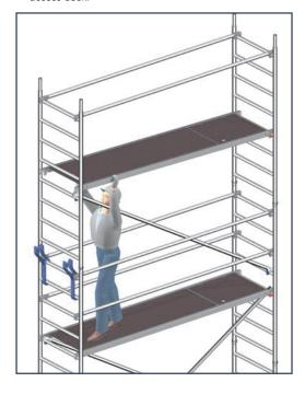
2 Swing ladder frame with rear guardrail upwards and fit into place.
