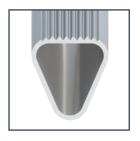
Rungs and steps made of high-strength and closed extruded sections without a longitudinal weld, for high load-bearing capacity. They are quadruple-folded in the stiles. The shape of the triangular rung ensures that it cannot turn, and the folding ensures high lateral stability of the ladder. The heavily grooved tread areas of the rungs and steps ensure a very sure footing.
