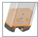
The Layher Combigrip ladder foot is made of a 2-component plastic: a hard inner section (orange) for secure mounting inside the stile, and a soft outer covering (black), non-slip on every floor surface. Easy retrofitting of cross-pieces - for compliance with the DIN EN 131 which starting on january 1, 2018 will specify a crosspiece for simple ladders of 3 metres and more length.
